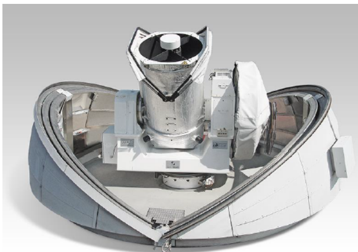
Figure 3.7.: ZIMLAT telescope which is used as the main telescope for photometry observations at Zimmerwald Observatory.
