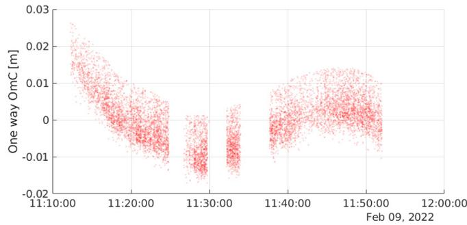
The results show that we can improve the residuals, however, one should notice the slight trend on them. This trend may be further removed if we modelled it as variations in the coordinates of the satellite, i.e. the orbit. Additionally, if there are available subsequent passes, we can check the consistency of the estimated range and time bias if we use the same set of ephemerides.
