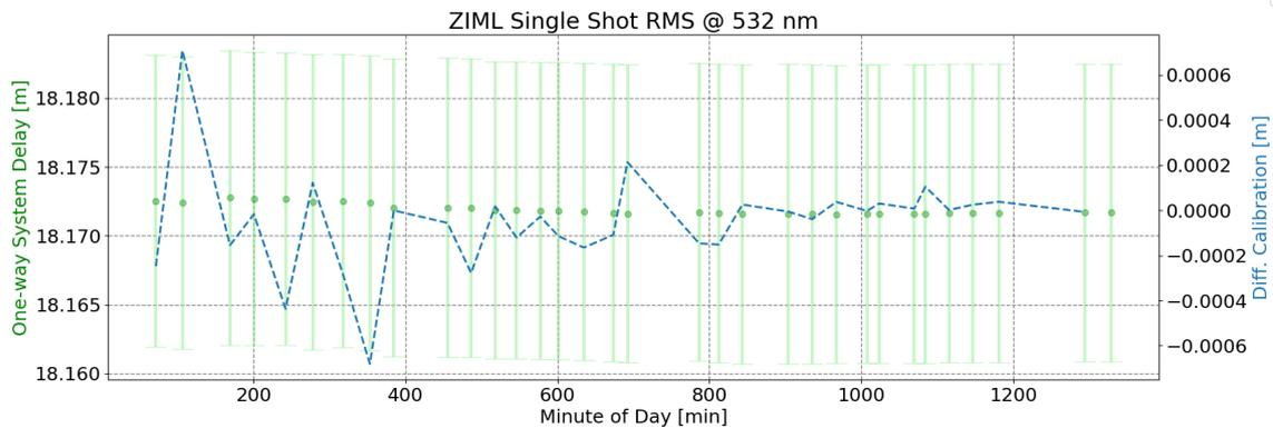
From such a historical set, we can verify certain aspects such as the agreement between the pulse width and the scattering of the single shot measurements, besides the stability of the system delays over time. Note that ideally, we would request potential sensors undertaking the V&Q procedure to provide a longer time span analysis to have a more representative figure.
