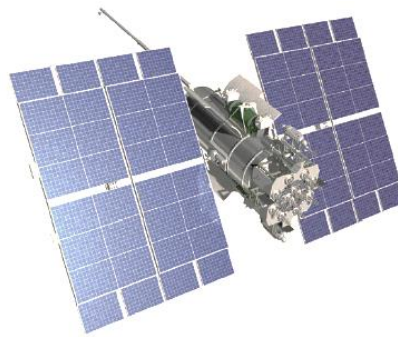
Fig. 2. Illustration of one of the first generation of GLONASS satellites (taken from [4]).
