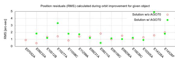
Fig. 6 - Position residuals (RMS) as calculated during AIUB's orbit improvement routine performed with CelMech tool. Plotted are solutions when AGO70 system data were not included to the processing (red) and were they were included to the processing (green).
