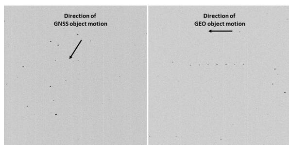
Fig. 4. Frames containing composites of images for GPS satellite (10022A) (left, a composite of 4 frames) and object E16022A (right, a composite of 7 frames) acquired by the AGO 70cm telescope during sidereal tracking. Exposures of 0.1s / R filter and 0.2s / R filter, respectively, were used.
