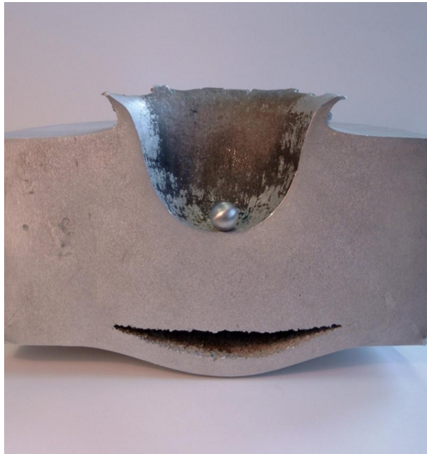
Figure 1.3: Damage caused by an object of a few millimeter in diameter that impacted a sheet of metal at hyper-velocity. http://www.esa.int/Our_Activities/Operations/Space_Debris/Hypervelocity_impacts_and_protecting_spacecraft . Accessed on 17/11/2016.
