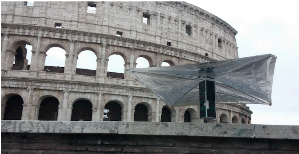
Fig 2. A full scale mockup of the 3U CubeSat URSA MAIOR with deorbit sail deployed.
