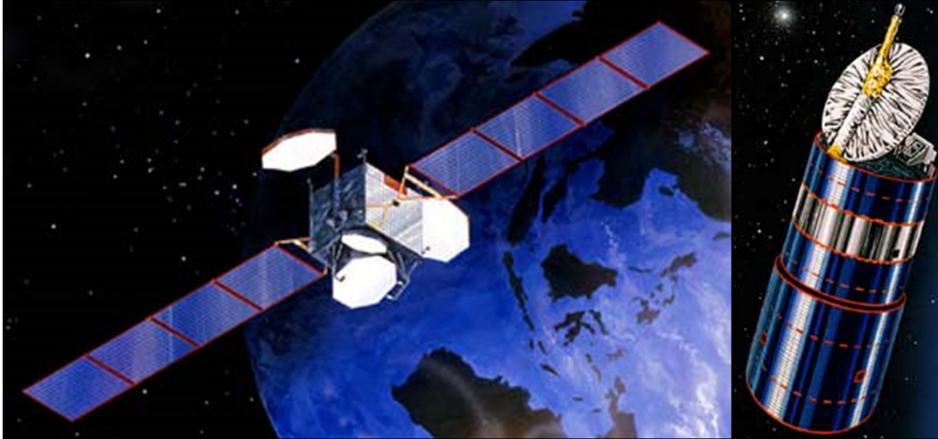
Fig. 1: (Images courtesy of Gunter's Space Page) An example box-wing (left) and cylindrical (right) geostationary satellite.
