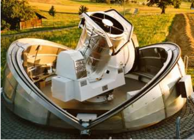
Figure 1. AIUB's 1-meter ZIMLAT telescope dedicated to the photometric and astrometric measurements
