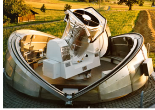
Figure 3. AIUBs 1-meter ZIMLAT telescope dedicated to the photometric and astrometric measurements.
