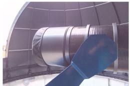
Fig. 1. New 50-cm telescopes ORI-50ML with field of view 2 degrees in Naucnniy-3, Crimea
