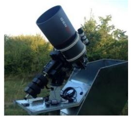
Fig. 3. New 30 cm telescope GenonMax with field of view 4.7 degrees in Nauchniy-1, Crimea
