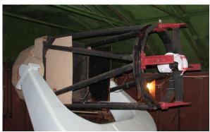
Fig. 2. Upgraded 80 cm telescope K-800 with field of view 55 minutes in Terskol, North Caucasus
