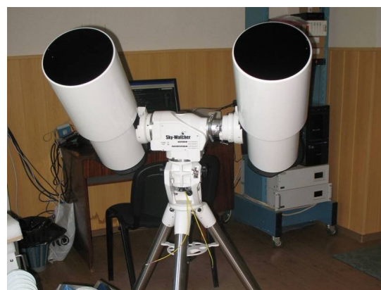
Fig. 7: Twin VT-18c telescope with 18-cm aperture for future observatory at Macon (Argentina). Summary field of view is 14x7 degree for two 36x36-mm CCD-chips.
