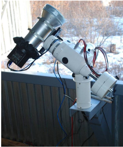
Fig. 4: VT-53e telescope with 12.5-cm aperture of JSC Vimpel in Blagoveschensk. Field of view is 12.3x8 degree for 36x24-mm CCD-chip.
