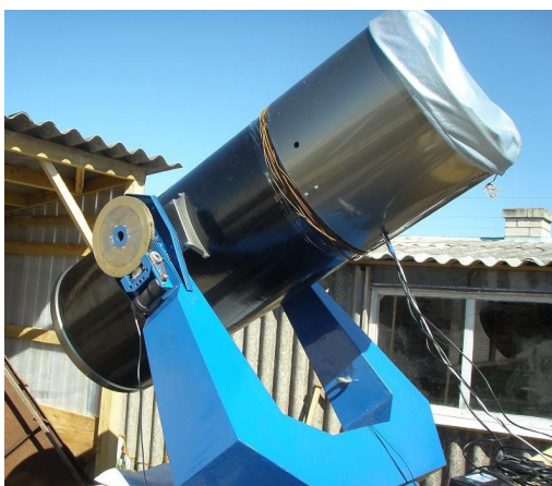
Fig. 9: ORI-50M telescope with 50-cm aperture in for future observatory in Andrushivka. Field of view is 2.5x2.5 degree for 50x50-mm CCD-chip.
