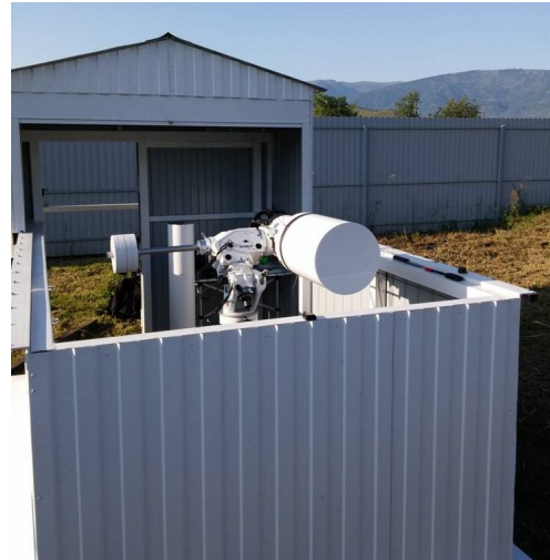
Fig. 5: VT-78a telescope with 19.2-cm aperture of NCT Ltd in new observatory at Multa (Altai republic) JSC Vimpel in Blagoveschensk. Field of view is 7x7 degree for 36x36-mm CCD-chip.
