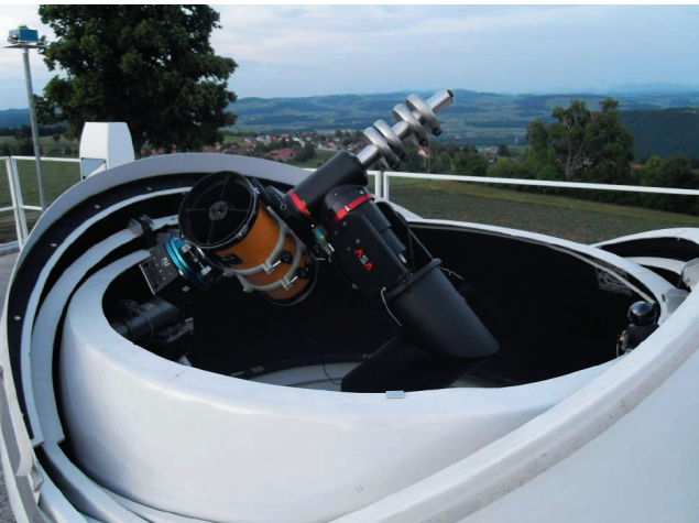
Fig. 2. AIUB's 0.18-meter ZimSMART telescope dedicated to the wide-field GEO surveys.
