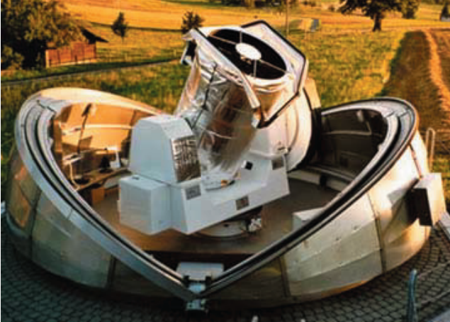
Fig. 1. AIUB's 1-meter ZIMLAT telescope dedicated to the photometric and astrometric measurements.
