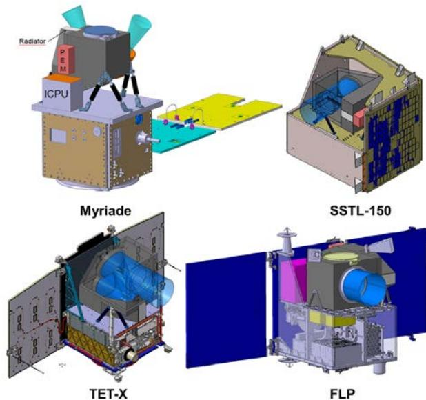
Fig. 6: Accommodation of the SBSS demonstrator instrument on different micro-sat platforms.
