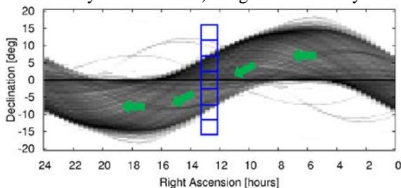
Fig. 2: Density plot of the GEO population and step-and-stare pointing pattern for the telescope FOV.
