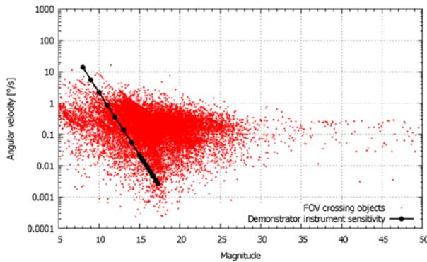
Fig. 8: Sensitivity limits of the SBSS demonstrator instrument. Objects below the curve can be detected.
