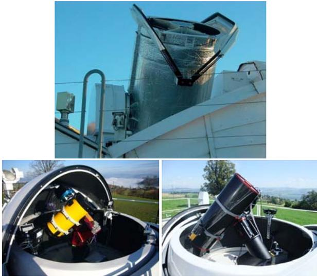
Figure 1: ZIMLAT 1-m telescope (top), ZimSMART 0.18-m (bottom left), and ZimSMART-2 0.3-m telescope (bottom right)
