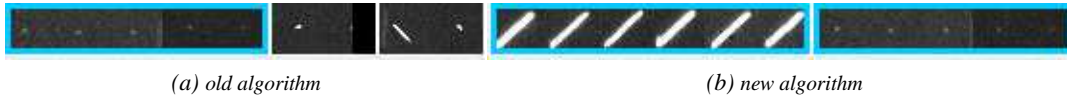
Figure 6.17: Less erroneous tracklets are linked by the new algorithm, in addition, images of an object in a high inclination orbit is linked.
