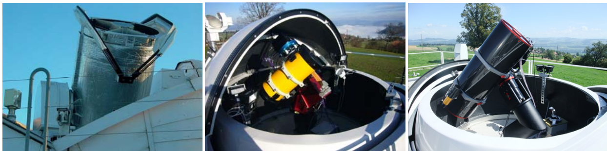
Figure 1: ZIMLAT 1-m telescope (left), ZimSMART 0.18-m (middle), and ZimSMART-2 0.3-m telescope (right).
