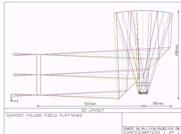
Figure 5. Optical design of the imaging elements.
